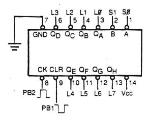
2. Turn all logic switches to off. Turn on power. D1 should light.
