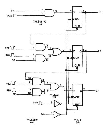
FIGURE 7-21. 74174 PIPO Shift Register.
